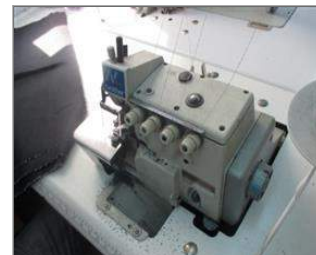
Photo of the personal protection equipments (if applicable) Over-Lock Machine with Eye Guard.JPG
